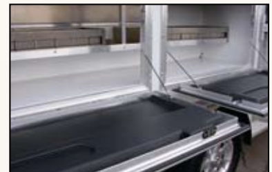
Full Access To Horizontal Compartments Shown With Optional Divider Bins
